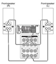
Connect the jacks on the Lo (or Hi) side of the front speakers to the FRONT SPEAKERS A jacks, and connect the jacks on the Hi (or Lo) side of the front speakers to the SURROUND BACK SPEAKERS terminals. Make sure that metal fittings of Hi/Lo attached to the speakers have been removed from the speakers. Not doing so may cause a malfunction of the receiver.
